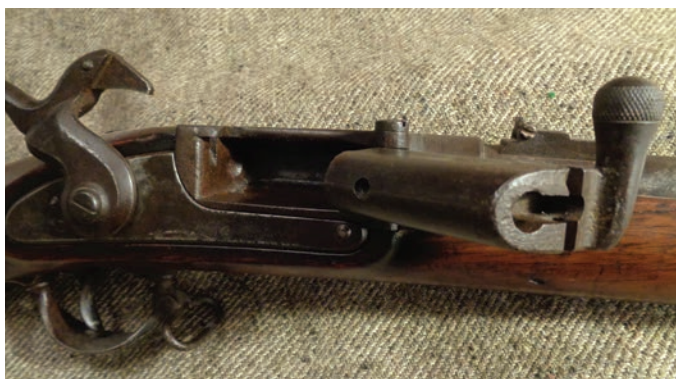
FIG 15. The authors conducted exhaustive tests to determine just how prone to jams the Needham conversion rifles really were. While some Needhams chambered cartridges satisfactorily, far more of them tended to jam. Courtesy of the author.
