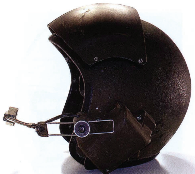
FIG 3. U.S. Army T56-6 Combat Vehicle Crewman helmet. The visor housing assembly from an SPH-4 flight helmet has been attached to this helmet for an eye shield. Author's collection.
