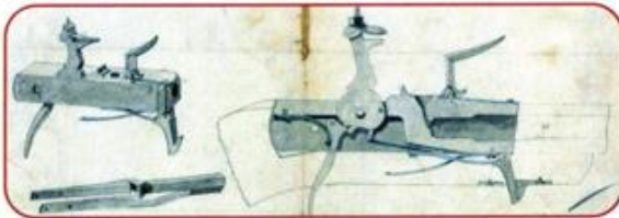
A drawing included in John Hall's original 1811 patent for what would become the M1819 Hall Rifle illustrates how the central breechblock is configured, having a chamber, hammer, frizzen, trigger, locking lever, trigger spring, mainspring and lever spring.
